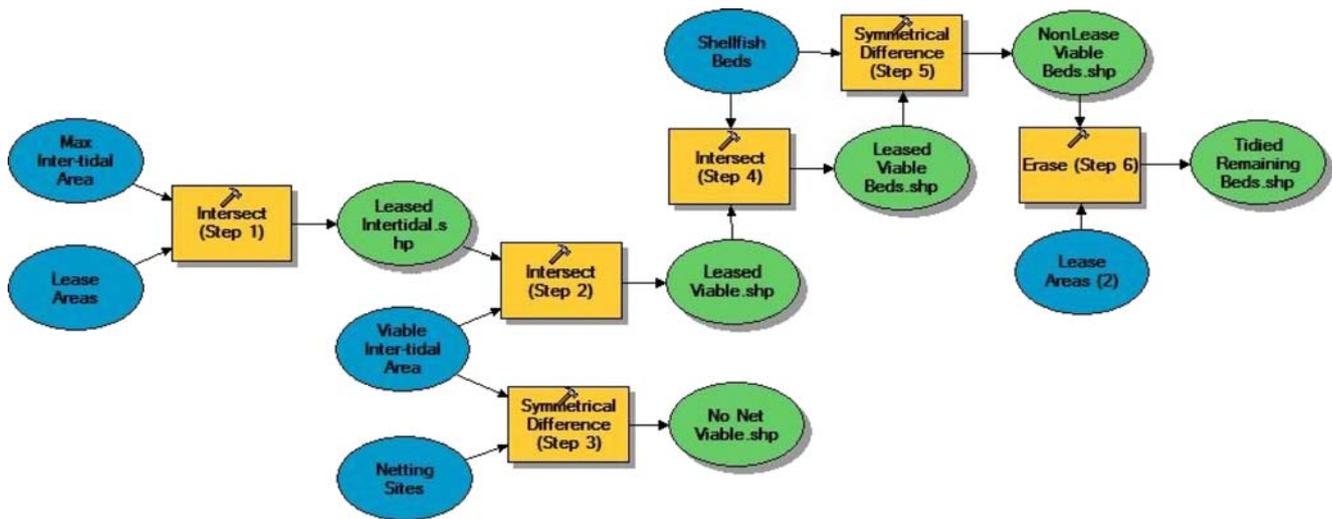
**Fig. 4** A full schematic of the spatial analysis model. Blue ovals represent input layers, green ovals represent outputs, and yellow rectangles represent operations
