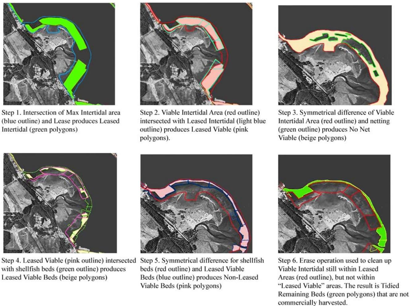
**Fig. 5** Application of the spatial analysis model as outlined in Fig. 4
